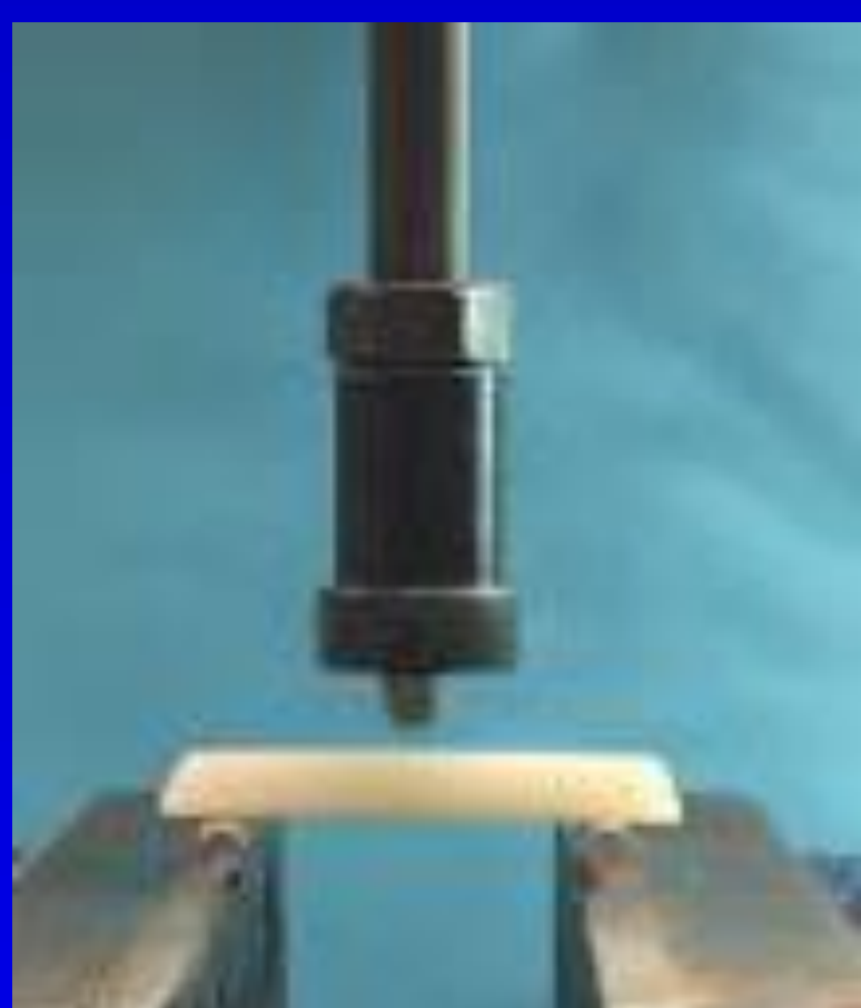
Three-point bending test set up
